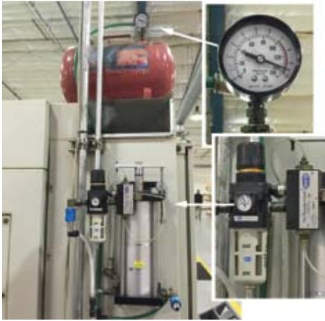
The job at hand for this machine center was to produce pneumatic valve bodies. The problem? Inadequate air pressure. Because of the extreme distance away from the factory's main compressor, pressure at the machine had dropped too low for its pneumatic vise to hold parts securely during a vital thread milling operation that was creating 1/4 NPT ports.
